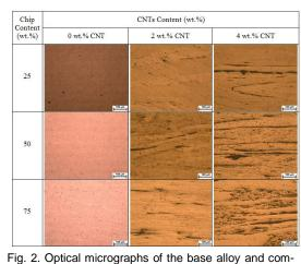
Fig. 2. Optical micrographs of the base alloy and composites with different amounts of Al chips in the range of 25–75 wt%.
